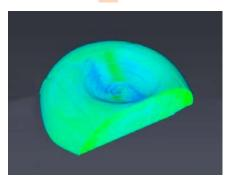
Collapse of a drop of liquid suspension ( $\emptyset$  = 1.48 mm) during drying: visualization of the solid accumulation (dark green) around the edges.
